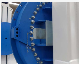
Blocco meccanico del carrello folle Mechanical lock of the slave carriage
