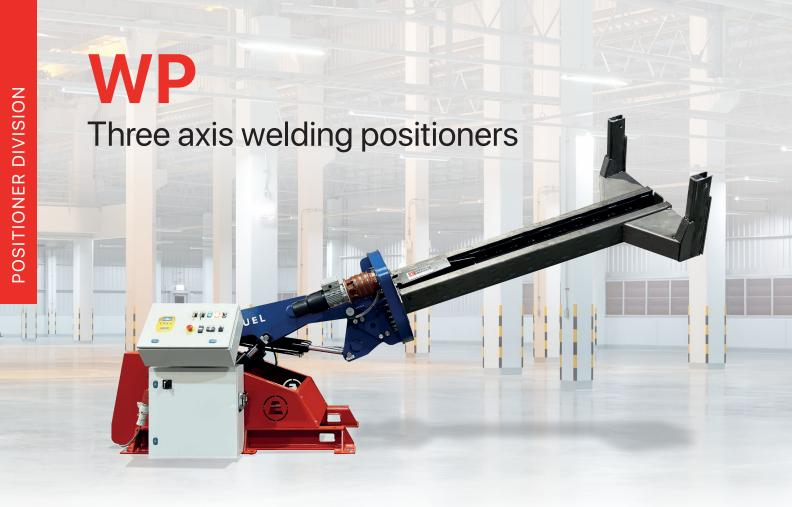
The **WP** is a three axis welding positioner that allows the lifting and the rotation of any of work piece during welding and assembly operations. Ergonomic positioners are used during welding and assembly operations of big work pieces that are manufactured by companies of all sectors. The ergonomics, technical characteristics and functional flexibility allow you to increase productivity and efficiency by minimizing the handling of the product on which it is necessary to work on.
